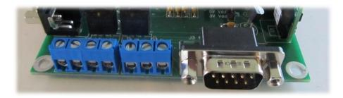
Limit switches should be normally (non-limit condition) closed to ground. The board has built in 10K pull up resistors to Vdd. When a limit is hit, the switch should open and the controller will see a logic high. Input 13 can be used for any unspecified input to the controller. It also has a pull up resistor.
