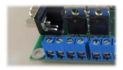
Up to 2 external relays can be controlled power via on board MOSFETs. The MOSFETs should be able to handle just about any 24V relay coil, but be careful that the total current from the steppers and the relays does not exceed the maximum of 5A for the board. The 24V terminal is always on and the return/ground terminal is switched to ground by the MOSFETs. A logic high on pin 1 or pin 8 of the J1 25 pin control connector activates the circuit
