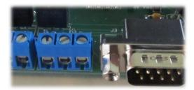
This terminal block can power a 5V or 24V fan. It can also be used to power light current off board accessories. Be sure not to exceed the 5A maximum current on the 24V power connector.
