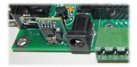
This connector is for the 24V input power of the board. The center pin is positive and the outer ring is ground. Double check the voltage before applying. Reverse voltage will destroy many parts on the board. Use a twisted pair of 18-22 AWG wires or coaxial shielded cable for this. The connector is rated for 5 amps continuous current. The mating connector is a standard 2.5mm x 5.5mm power connector.
