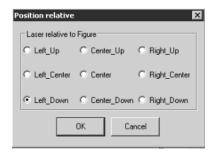
b. In the dialog that appears, select Left\_Down. This means that, at the beginning of a job, the start point (origin) is at the Left Down (bottom) of the output. In other words, the head will move UP and RIGHT to actually draw the output.
